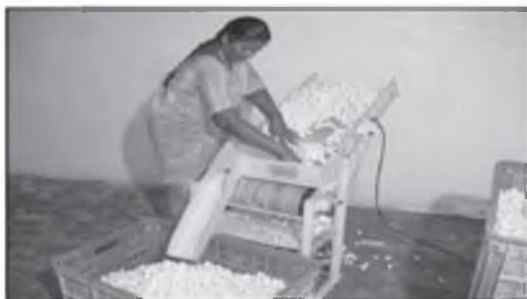
22-rasm. Pillalarni losdan tozalaydigan dastgoh
