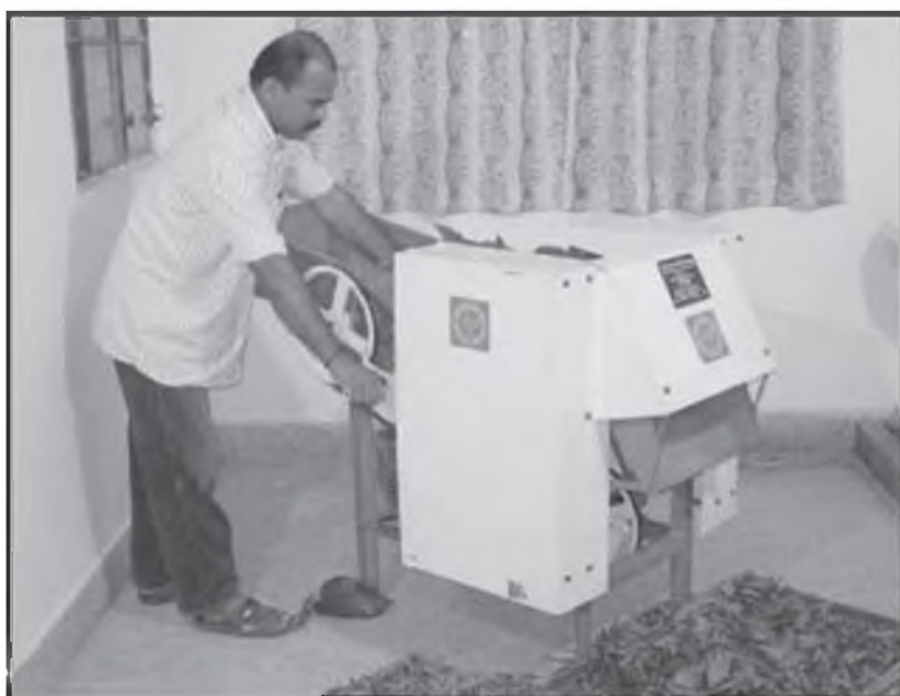
19-rasm. Avtomatik barg to'g'ragich asbobi
