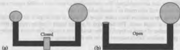
FIGURE 2.7a,b Equilibrium state of two bubbles of different radii (see text).
