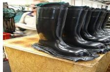
Compression molded (cured) rubber boots before the flashes are removed.
