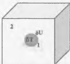
Figure 12.1 Thermal fluctuations in the equilibrium state. We consider a fluctuation that results in a flow of energy \delta U from one part to the other, causing the temperatures to change by a small amount \delta T .
