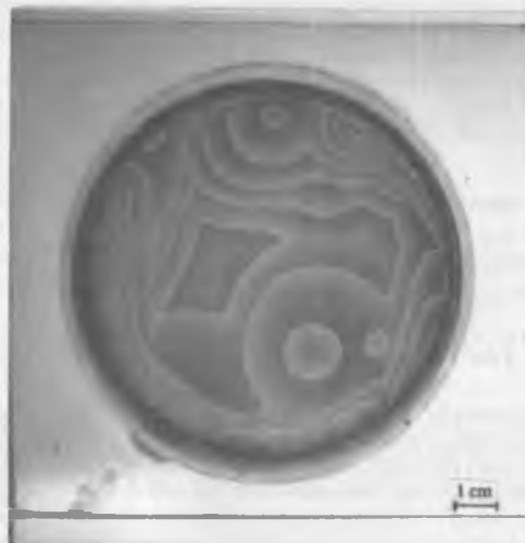
Figure 19.12 Traveling waves in the Belousov-Zhabotinsky reaction.
