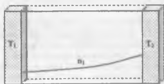
Figure 16.5 Thermal diffusion: a temperature gradient and the consequent flow of heat causes a concentration gradient.
