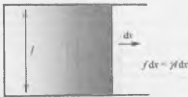
Figure 5.5 Energy is required to enlarge a surface of a liquid. The force per unit length is \gamma .
