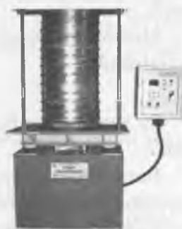
68-rasm. Zamonaviy KP-109.2 modeli sim g'alvir.
