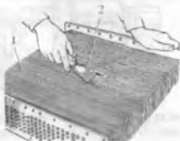
20.37-rasm. Radiator plastinkalarini to'g'irlash: 1-radiator; 2-to'g'irlagich.
