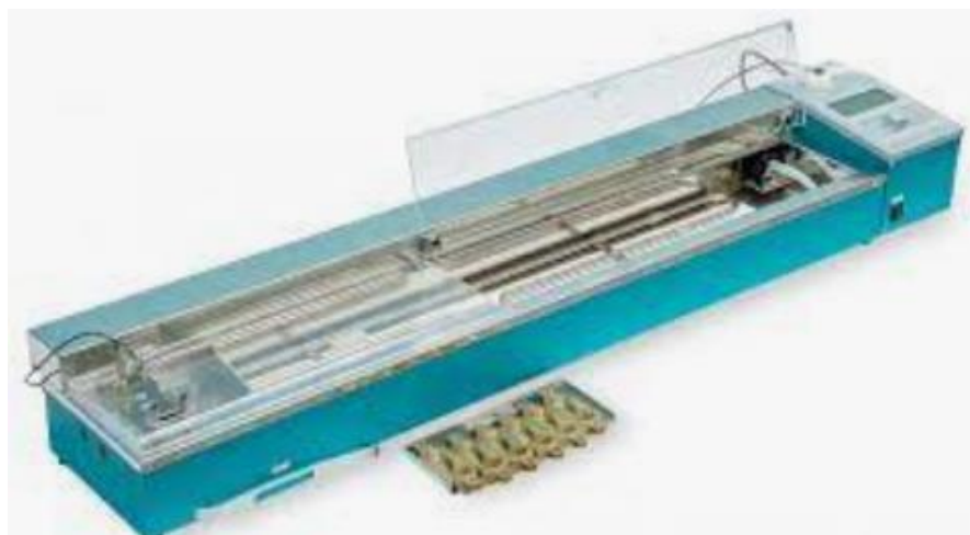
12.3-rasm. Duktilometr- bitumlarning cho'ziluvchanligini aniqlash jihozi
