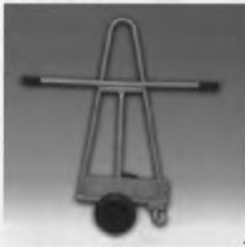
2.8-rasm. GKQ larni tashish uchun transport vositalari: a – ikki g'ildirakli KNAUF aravachasi; b – GKQ ni o'tkazish uchun dastak.
