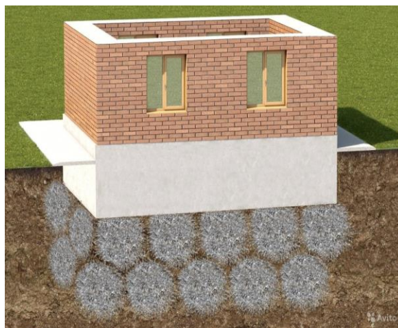
4.13-rasm. Grunt zaminining mustahkamlanmagan (a) va mustahkamlangan sharoitidagi binoning holati
