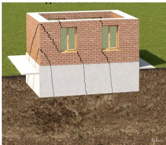
4.13-rasm. Grunt zaminining mustahkamlanmagan (a) va mustahkamlangan sharoitidagi binoning holati
