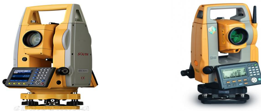
3.4-rasm. Sokkia va Topcon rusmli taxeometrlar
