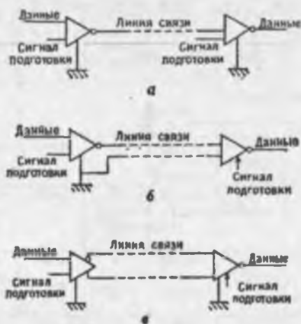
1.15-rasm. Ketma-ket shinalarning topologiyasi: a—RS 232, б—RS 422, в—RS 423.
