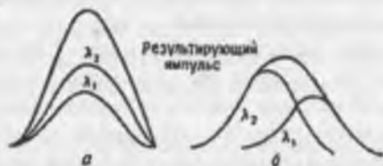
1.27-рasm. Material dispersiya tufayli impulsning kengayishi: a — dastlabki impuls, b — chiqish impuls. ■
