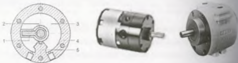
3.2.20-rasm. Plastinali (shiberli) aylanuvchi pnevmodvigatel.
