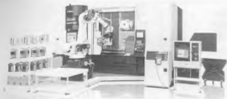
2.1.8-rasm. E-BOT 720 robotlashtirilgan yacheyka
