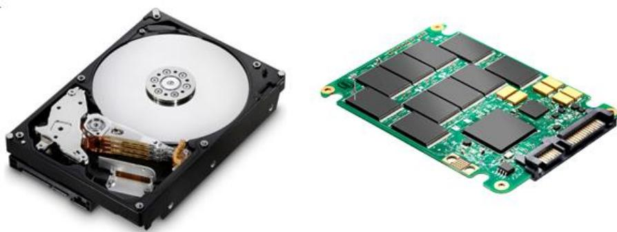
1.8-rasm. HDD va SSD vinchesterlari
