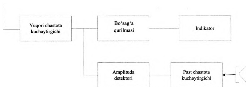
10.4-rasm. Elektromagnit nurlanish indikatorining sxemasi.
