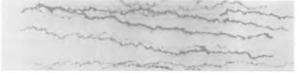
Fig. 1. Sample trajectories of sedimenting mercury droplets measured by Ivar Nordlund in 1914 with his moving film technique, time increases to the right. 6 The jiggly motion of the droplets superimposed onto the deterministic sedimentation shows the Brownian motion of the droplets.
