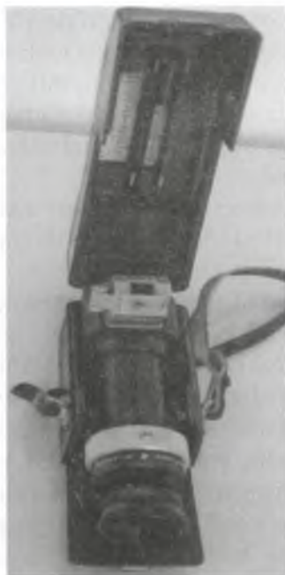
2.24-rasm. IRF-464 rusumli ko'chma refraktometr.
