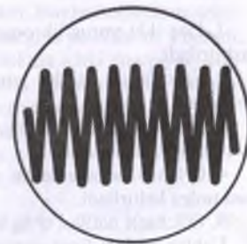
2.38-rasm. Yoritgich spiral tolasining linzadagi tasviri.
