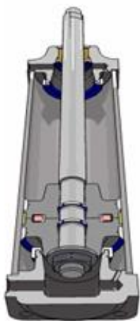
9.14-rasm. 3D-formatdagi pnevmatik porshenli silindr qirgimi
