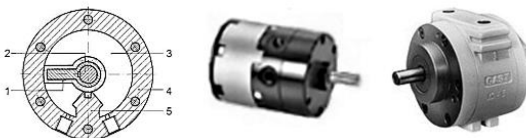
9.25-rasm. Plastinali (shiberli) aylanuvchi pnevmodvigatel.
