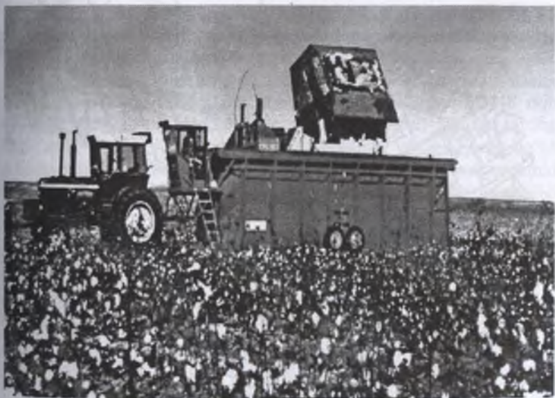
42-rasm. Paxta terish kombaynidan chigitli paxtani modulga ortish jarayoni.
