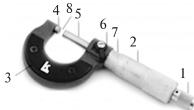
2-rasm. Mikrometrning tuzilishi.
