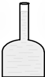
2-rasm. Eng oddiy piknometr.
