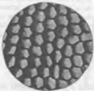
II.56-rasm. Rayshan kataksimon tuzilishli kristallanish fronti sirtining tashqi ko'rinishi (qalay-qo'rg'oshin tizimi).
