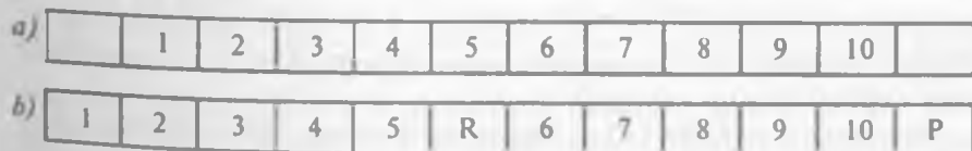
11.9-rasm. 10B1R1P turdagi liniya kodini shakllanish sxemasi:
