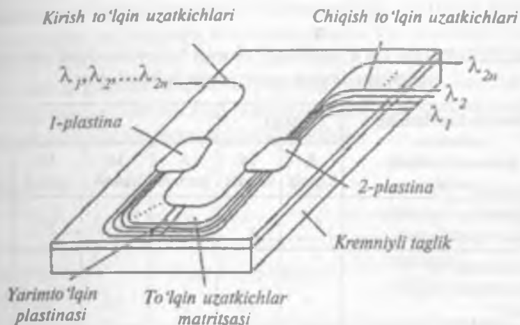
9.5-rasm. Tolali optik multipleksorning tuzilishi
