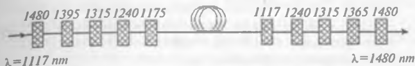
14.7-rasm. VKR lazerning tuzilish sxemasi [6]
