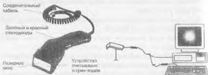
31-rasm. MS-951 qo'lli skaner va uning personal kompyuterga ulanishi 5 .
