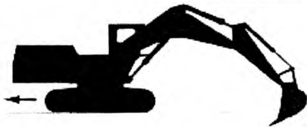
3.5-rasm. Ekskavator kovushini zaminga kuch bilan botirishning oqibati
