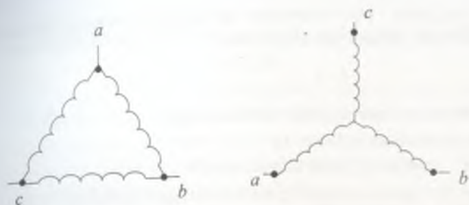
4.9-rasm. Stator chulg'amini ulash sxemalari
