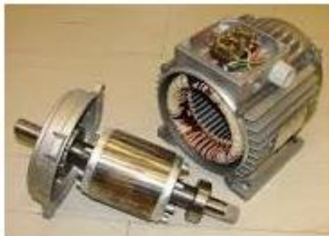
1.20-rasm. 4A rusumli asinxron motor.
