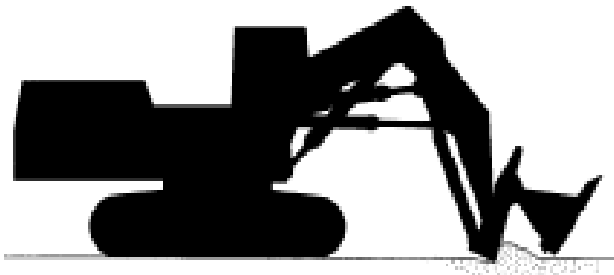
12.6-rasm. Ekskavator kovshini orqa tomoni bilan zaminni tekislashning salbiy oqibati
