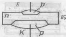
III.66-rasm Qotishmali tranzistor tuzilmasi
