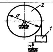
**8.4.10.** Tishlar soni  $Z_1=26$  va  $Z_2=78$ , radiusi  $r=10\text{sm}$  bo'lgan g'ildiraklarga osilgan yukni  $v=90\text{sm/s}$  tezlik bilan tortadi. 1 g'ildirakning aylanish chastotasi  $n_1(\text{ayl/min})$ ni toping. (258)
