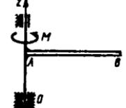
**16.1.16.** Dvigatel rotoriga  $M=100(1-\omega/200)$  juft kuch momenti ta'sir etib, uni ishga tushirsa, rotorning inersiya momentini  $2\text{kg}\cdot\text{m}^2$  hisoblab, rotor burchak tezlanishining maksimal qiymatini aniqlang. (50)
