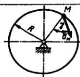
**8.3.16.** Qo'zg'almas o'q atrofida aylanayotgan diskning  $M$  nuqtasi  $8\text{m/s}^2$  tezlanishga ega bo'lsa, uning radiusini  $R=0,4\text{m}$  va  $\gamma=30^\circ$  deb, diskning burchak tezlanishini toping. (10)
