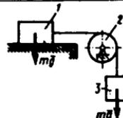
**17.3.14.** Massasi  $m=0,6\text{kg}$  dan bo'lgan 1 va 3 yuklar ip yordamida blok orqali bog'langan bo'lib  $a=3\text{m/s}^2$  tezlanish bilan harakat qilsa, 2 blokning massasini hisobga olmay, blok sharnirida hosil bo'lgan reaksiya kuchini toping. (5,78)
