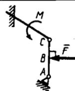
**3.2.8.** Uzunligi  $CD=2\text{m}$  bo'lgan sterjenga momenti  $M=400\text{N}\cdot\text{m}$  li juft kuch ta'sir qilsa,  $C$  sharnirdagi reaksiya kuchining gorizontal tashkil etuvchisi  $X_C$  ni toping. (200)
