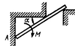
**2.4.20.** AB to'sin devorga qistirib mahkamlangan CD sterjenga tiralgan. Agar to'sining uchiga  $F=4\text{N}$  bo'lgan kuch ta'sir etsa, masofa va burchaklarini  $AB=2\text{m}$ ;  $BD=1/3 AB$ ,  $\alpha=60^\circ$  hisob-lab, CD sterjenda hosil bo'lувчи reaksiya kuchini toping. (5,20)
