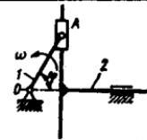
**14.1.16.** Krivoship-polzunli mexanizmning  $A$  va  $B$  nuqtalarining tezlanishi  $a_A=10\text{m/s}^2$  va  $a_B=14\text{m/s}^2$  bo'lib, massasi  $m=5\text{kg}$  bo'lgan, bir jinsli sterjen shaklidagi shatun  $AB$  ga ta'sir qiluvchi tashqi kuchlar bosh vektorining  $\varphi=180^\circ$  holatdagi miqdorini toping. (60)
