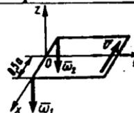
**12.4.10.** Mexanizmnинг 3 diskni 2 dastakka nisbatan  $\omega_3=0,5\text{rad/s}$  burchak tezlik bilan, 2 dastak esa 1 dastakka nisbatan  $\omega_2=0,2 \text{ rad/s}$  burchak tezlik va 1 dastakning burchak tezligi  $\omega_1=0,1\text{rad/s}$  bilan aylansa,  $\bar{\omega}_2 \parallel \bar{\omega}_3 \parallel Ox$  deb, 3 disk absolut burchak tezligining qiymatini toping. (0,316)
