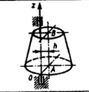
**16.1.21.** Devorga qistirib mahkamlangan  $OA$  konsol to'sinining uchiga rotor o'rnatilgan bo'lib, u tiklovchi moment  $M_z=-\pi^2\varphi$  ta'sirida  $\varphi=3\sin(\pi/4)t$  qonun bilan burilma tebranishda bo'lsa, rotorning  $Az$  o'qiga nisbatan inersiya momentini hisoblang. (16)
