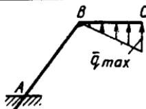
**2.3.22.** Qistirib mahkamlangan to'sinning qancha  $\ell$  qismiga intensivligi  $q_{\max}=10\text{N/m}$  li taqsimlangan kuchlar ta'sir etsa,  $A$  tayanchning reaksiya kuchi  $R_A=10\text{N}$  ga teng bo'ladi? (2,0)
