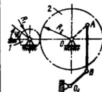
**8.4.14.** Radiuslari  $R_1=0,3\text{m}$ ,  $R_2=0,9\text{m}$  bo'lgan tishli g'ildiraklarga bog'langan krivoshipning o'lchamlari  $O_1M=0,3\text{m}$ ,  $OA=O_1B$  va  $AB=OO_1$  bo'lib, 1 g'ildirak o'zgarmas  $\omega_1=6\text{rad/s}$  burchak tezlik bilan aylansa, krivoship M nuqtasining tezlanishini toping. (1,2)
