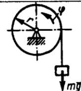
**17.1.2.** Massasi  $m=60\text{kg}$  bo'lgan yuk ip yordamida g'altakka osilgan. Agar g'altakning radiusi  $r=0,4\text{m}$  bo'lib,  $\varphi=0,6t^2$  qonun bo'yicha aylansa, ipning taranglik kuchini toping. (617)
