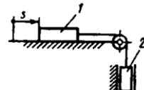
**20.5.13.** Mexanik sistema massasi  $m=20\text{kg}$  bo'lgan 1 jism va aylanish o'qiga nisbatan inersiya momenti  $J_0=2\text{kg}\cdot\text{m}^2$  ga teng 2 silindr dan iborat. Agar silindrning radiusi  $r=0,2\text{m}$  bo'lib, momenti  $M=20\text{N}\cdot\text{m}$  li juft kuch ta'sirida aylansa va sistemaning kinetik energiyasi  $T=35\dot{s}^2$  ga ega bo'lsa, 1 jismning tezlanishi  $a_1$  ni aniqlang. (0,470)
