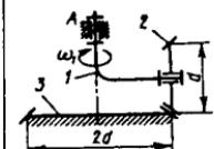
**12.2.3.** 1 disk ikkita aylanma harakatda ishtirok etadi. Birinchidan disk 2 dastak o'z o'qi atrofida  $300\text{ayl/min}$  chastota bilan, 2 dastak esa 3 podshipnik atrofida  $\omega_2=10\text{rad/s}$  burchak tezlik bilan aylanadi. Diskning absolut burchak tezligini toping. (33,0)
