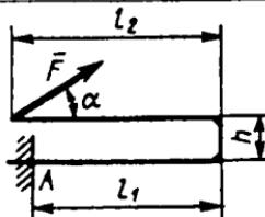
**2.4.39.** Devorga qistirib mahkamlangan to'singa sim arqon yordamida  $F=50\text{kN}$  qiymatli gorizontal kuch ta'sir etib,  $h=0,5\text{m}$  bo'lsa, A tayanchdagi momentning qiymatini  $\text{kN}\cdot\text{m}$  da toping. (25,0)
