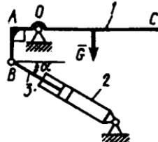
**2.4.31.** Avtomashinanining kuzovi  $G=10\text{kN}$  og'irlikka ega bo'lib, 2 kuch gidrosilindr yordamida muvozanatda ushlab turibdi. Agar masofa va burchaklar  $\ell=3\text{m}$ ,  $b=1,2\text{m}$ ,  $AO=1\text{m}$ ,  $\alpha=30^\circ$  bo'lsa, gidrosilindr 3 dastagiga ta'sir etuvchi kuchni aniqlang. (11,5)
