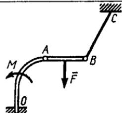
3.2.3. O'lchamlari  $AB=2\text{m}$  va  $BC=0,5\text{m}$  bo'lgan sterjenlardan iborat sistemaga momenti  $M=800\text{N}\cdot\text{m}$  li juft kuch ta'sir etsa,  $C$  tayanchdagi reaksiya momentini aniqlang. (200)
