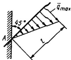
**2.3.23.** Qistirib mahkamlangan ramaning  $\ell=1\text{m}$  li qismiga intensivligi  $q$  qancha bo'lgan taqsimlangan kuchlar ta'sir etsa,  $A$  tayanchning reaktiv momenti  $M_A=200\text{N}\cdot\text{m}$  ga teng bo'ladi? (4,0)
