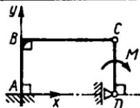
**3.2.9.**  $B$  sharnir orqali bog'langan sterjenlarga  $F_1=60\text{N}$  va  $F_2=50\text{N}$  li kuchlar ta'sir etsa,  $A$  tayanchdagi moment miqdorini aniqlang. (240)
