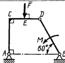
**3.2.14.** O'lchamlari  $BC=2AB$  bo'lgan  $AC$  sterjenga  $F=600\text{ N}$  kuch ta'sir etsa,  $C$  sharnir reaksiya kuchining vertikal tashkil etuvchisini toping. (200)
