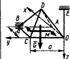
**5.6.10.** O'lchamlari  $a=20\text{sm}$  bo'lgan bir jinsli plita  $G=400\text{N}$  og'irlikka ega. Agar plita shaklda ko'rsatilgan bog'lanishlar vositasida muvozanatda bo'lib,  $\alpha=61^\circ$ ,  $\beta=44^\circ$  va  $\gamma=60^\circ$  bo'lsa,  $AB$  arqonning taranglik kuchini,  $Ox$  o'qiga nisbatan moment tenglamasini tuzib toping. (400)
