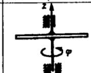
**16.1.5.** Massasi  $m=60\text{kg}$ , radiusi  $R=1,41\text{m}$  bo'lgan bir jinsli silindrning harakat tenglamasi  $\varphi=t^3-5t^2$  bo'lsa,  $t=2\text{s}$  dagi jismga ta'sir etuvchi tashqi kuchlarning bosh momentini hisoblang. (119)
