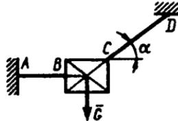
**1.2.13.** Ikki sterjen  $AC$  va  $BC$  o'zaro  $C$  sharnir yordamida bog'langan. Agar  $C$  sharniriga  $D$  blok orqali og'irligi  $12\text{N}$  bo'lgan yuk osilib,  $\alpha=60^\circ$  bo'lsa,  $BC$  sterjenning reaksiya kuchini toping. (-6)
