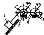
**8.4.13.** Radiuslari  $R_1=0,3\text{m}$ ,  $R_2=0,9\text{m}$  bo'lgan tishli g'ildiraklarga mahkamlangan krivoshipning o'lchamlari  $O_1B=OA=0,6\text{m}$  va  $OO_1=AB$  bo'lib, 1 g'ildirak  $\varphi_1=2t^3$  qonun bo'yicha aylansa,  $t=2\text{s}$  paytda krivoship B nuqtasining tezligini aniqlang. (4,8)
