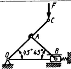
3.3.8. Krivoship-polzunli mexanizm  $F_1=1$  kN va  $F_2$  kuchlar ta'sirida muvozanatda bo'lsa,  $OA=AC=0,3$  m va  $\alpha=45^\circ$  deb,  $OAC$  krivoship va  $AB$  shatunning o'zaro ta'sir kuchini kN da aniqlang. (1,41)
