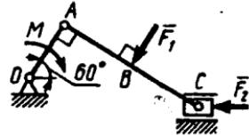
**3.3.10.** Kulisali mexanizm  $F_1=1\text{kN}$  va  $\bar{F}_2$  kuchlar ta'sirida muvozanat holatida bo'lib,  $OA=0,5\text{m}$ ,  $OB=1,2\text{m}$ ,  $\varphi=30^\circ$ ,  $\alpha=60^\circ$  bo'lsa, 1 vtulkaning 2 vertikal sterjenga bosim kuchini  $\text{kN}$  da aniqlang. (2,08)
