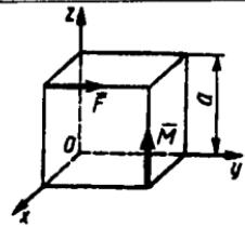
**5.3.11.** O'lchamlari  $a=1\text{m}$  va  $\alpha=60^\circ$  bo'lgan ramaga miqdori  $F=100\text{N}$  kuch va momenti  $M=50\text{N}\cdot\text{m}$  li juft kuch ta'sir etadi. Ularning  $O$  nuqtaga nisbatan bosh momentining modulini toping. Bunda  $\bar{F} \parallel Oz$  va  $\bar{M} \parallel Ox$ . (100)
