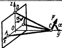
**1.4.4.** Uchta sterjen  $AD$ ,  $BD$  va  $CD$  sharnirlar bilan mahkamlangan bo'lib,  $D$  sharniriga  $20\text{N}$  li yuk osilgan bo'lsa,  $CD$  sterjenning zo'riqishini toping ( $\alpha=45^\circ$ ). (-28,3)
