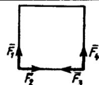
**2.2.3.** Kvadratning uchlariga to'rtta  $F_1=F_2=F_3=F_4=1\text{N}$  kuchlar ta'sir etsa, ularning bosh vektori miqdori nechaga teng? (2,0)
