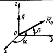
**5.4.13.** Koordinata boshini keltirish markazi deb olingan holda, bosh vektor  $\bar{R}$  va bosh moment  $\bar{M}_0$  ning koordinata o'qlardagi proyeksiyalari  $R_x=1\text{N}$ ,  $R_y=3\text{N}$ ,  $R_z=0$ ,  $M_x=5\text{N}\cdot\text{m}$ ,  $M_y=4\text{N}\cdot\text{m}$  va  $M_z=1\text{N}\cdot\text{m}$  berilgan.  $\bar{R}$  va  $\bar{M}_0$  vektorlarning skalar ko'paytmasini hisoblang. (17)
