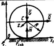
**16.2.16.** Massasi  $m=300\text{kg}$ , radiusi  $R=0,15\text{m}$  va inersiya momenti  $J_{cz}=3,4\text{kg}\cdot\text{m}^2$  bo'lgan silindr juft kuch momenti  $M=75\text{N}\cdot\text{m}$  ta'sirida qiya tekislikdan yuqoriga ko'tarilsa, ishqalanish kuchini  $F_{ishq}=255\text{N}$  deb, uning burchak tezlanishini aniqlang. (10,9)
