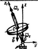
**16.3.3.** Inersiya momenti  $J_{zi}=0,001\text{kg}\cdot\text{m}^2$  bo'lgan pirildoq  $\omega_1=100\text{rad/s}$  va  $\omega_2=1,4\text{ rad/s}$  burchak tezliklar bilan muntazam pretsessiyada bo'lib,  $\bar{\omega}_1$  va  $\bar{\omega}_2$  larning orasidagi burchak  $\theta=5^\circ$  bo'lsa, uning og'irlilik kuchi  $\bar{G}$  ning  $O$  nuqtaga nisbatan momentini hisoblang. ( $1,22 \cdot 10^{-2}$ )
