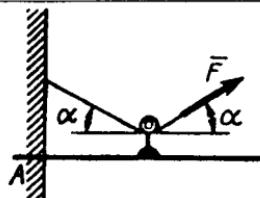
**2.4.41.** Yerga qistirib mahkamlangan, uzunligi  $AB=5,66\text{m}$  bo'lgan to'sinning uchiga  $F$  kuchi ta'sir etayotgan bo'lsa, A tayanchdagi reaksiya momenti  $M_A=56\text{kN}\cdot\text{m}$  ga teng bo'lsa,  $F$  kuchining qiymatini  $\text{kN}$  da toping. (14,0)
