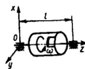
**17.4.21.** Rotor juft kuch momenti  $\bar{M}$  ta'sirida  $\omega=10\text{rad/s}$  burchak tezlik va  $\epsilon=60\text{rad/s}^2$  burchak tezlanish bilan  $Oz$  o'qi atrofida aylanadi. Agar rotoring markazdan qochma inersiya momentlari  $J_{xz}=0$ ,  $J_{yz}=5\cdot10^{-3}\text{ kg}\cdot\text{m}^2$  bo'lib, podshipniklar  $\ell=0,25\text{m}$  masofada bo'lsa,  $O$  podshipnikdagi dinamik reaksiya kuchini aniqlang. (2,33)
