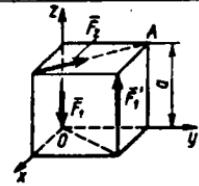
**5.3.14.** O'lchamlari  $b=2a=c=2\text{m}$  bo'lgan parallelepipedga  $\beta=\gamma=60^\circ$  burchak ostida  $F=26\text{N}$  kuch va  $M=13\text{N}\cdot\text{m}$  momentli juft kuchlar qo'yilgan.  $A$  nuqtani keltirish markazi deb, kuchlar sistemasining bosh momentini aniqlang. (13)
