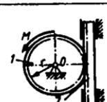
19.2.7. Radiuslari  $r_1=0,05\text{m}$  va  $r_2=0,1\text{m}$ ; aylanish o'qlariga nisbatan inersiya momentlari  $J_1=0,01\text{kg m}^2$  va  $J_2=0,02\text{kg m}^2$  bo'lgan shkivlar momenti  $M=0,15\text{N}\cdot\text{m}$  li juft kuch ta'sirida harakatga kelsa, 1 shkivning burchak tezlanishini aniqlang. (10)
