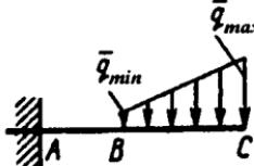
**2.3.20.** O'lchamlari  $AB=1\text{m}$ ,  $BC=2\text{m}$ ,  $CD=3\text{m}$  bo'lgan to'sin devorga qistirib mahkamlangan bo'lib, unga  $\bar{F}$  kuchi va intensivligi  $q_{\max}=20 \text{ N/m}$  bo'lgan taqsimlangan kuchlar ta'sir etib,  $A$  tayanchdagi reaktiv moment  $300 \text{ N}\cdot\text{m}$  ga teng bo'lishi uchun  $\bar{F}$  kuchining miqdori qancha bo'lishi lozim? (180)
