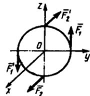
**5.2.12.** Mashina detalining to'rt tomoniga miqdorlari teng  $M_1=M_2=M_3=M_4=5\text{ N}\cdot\text{m}$  momentli juft kuchlar va  $Oyz$  tekisligida qiymati  $F=\bar{F}=100\text{ N}$  bo'lgan  $(\bar{F}, \bar{F}')$  juft kuch ta'sir etsa, juft kuchlar sistemasining teng ta'sir etuvchisining momentini toping. Bunda  $a=0,05\text{ m}$  va  $\bar{F} \parallel Oz$   $\bar{F}' \parallel Oz$  deb oling. (17,3)
