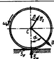
**22.4.5.** Massasi  $m=0,6\text{kg}$  bo'lgan disk  $\omega_0=2\text{rad/s}$  burchak tezlik bilan aylanib, massa markazi  $v_0=1,8\text{m/s}$  tezlikka ega holda vertikal devorga  $\alpha=45^\circ$  burchak ostida uriladi. Agar normal impulsning tiklash koeffitsiyenti  $k=0,55$  bo'lsa, normal impuls  $S_N$  ning qiymatini hisoblang. (1,18)
