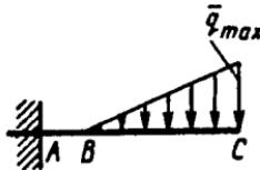
**2.3.19.** O'lchamlari  $AB=2\text{m}$ ,  $BC=6\text{m}$  bo'lgan to'sin devorga qistirib mahkamlangan bo'lib, unga intensivliklari  $q_{\max}=30 \text{ N/m}$  va  $q_{\min}=10 \text{ N/m}$  bo'lgan taqsimlangan kuchlar ta'sir etsa,  $A$  tayanchdagi reaktiv momentning miqdorini toping. (660)
