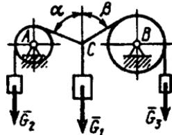
1.2.20. Og'irliklari  $\bar{G}_1$  va  $\bar{G}_2$  bo'lgan ikki yuk  $B$  sharnirga va  $A$  blokka ip vositasida osilgan. Agar  $G_2=90N$ ,  $\alpha=45^\circ$ ,  $\beta=60^\circ$  berilgan bo'lsa,  $BC$  ipning taranglik kuchini hisoblang. (73,5)
