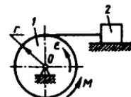
**17.3.17.** Vibrator ikki sinxron aylanuvchi pnevmoturbinalardan iborat bo'lib, ularning valiga  $r=10\text{sm}$  masofada  $m=0,5\text{kg}$  massalar o'rnatilgan. Agar trubinalar  $n=1000\text{ayl/min}$  chastotasi bilan aylansa, vibrator asosiga ko'rsatilayotgan eng katta dinamik zo'riqishni toping (kN). (1,10)
