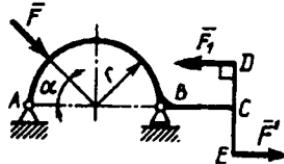
**2.1.8.**  $AB$  arkaga ( $\bar{F}_1, \bar{F}'_1$ ) juft kuch va  $\bar{F}$  kuchi ta'sir etadi. Agar kuchlarning miqdori  $F=4\text{N}$ ,  $F_1=2\text{N}$ , arka radiusi  $r=2\text{m}$ , juft kuch yelkasi  $CD=1,5\text{m}$  bo'lsa, ularning  $A$  nuqtaga nisbatan momentlarining yig'indisini aniqlang. (-11,0)
