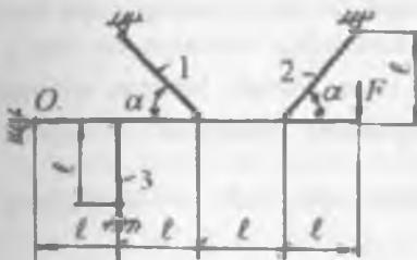
48 – rasm. Statik noaniq sterjenlar sistemasi
