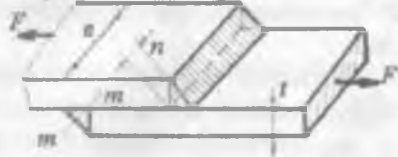
4.13-rasm. Ustma-ust payvandlash.
