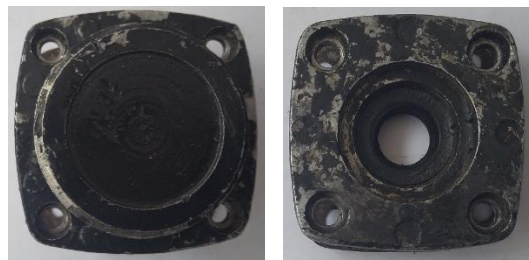
33-rasm. Chervyakli reduktor uchun podshipnik qopqoqi
