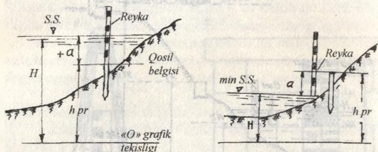
2.3-rasm. Suv sathini nol grafikka nisbatan o'lchash a – musbat sanoq (+ a ); b – manfiy sanoq ( -a ).
