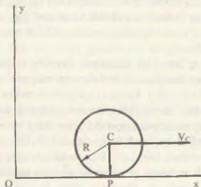
$$\bar{v}_p = \bar{v}_c + \bar{\omega} \times \bar{r} = 0$$
