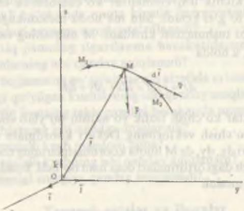
$\bar{F}$  kuchning Dekart o'qlaridagi proyeksiyalari.  $ds \neq 0$  bo'lganda  $0 < (\bar{F}^\wedge, \mathbf{v}) < 90^\circ$  bo'lsa,  $\delta A > 0$ ,  $90^\circ < (\bar{F}^\wedge, \mathbf{v}) < 180^\circ$  bo'lsa,  $\delta A < 0$  va  $\bar{F} \perp \mathbf{v}$  da esa  $\delta A = 0$  bo'lishi (10.2) formuladan kelib chiqadi. Kuchning  $M_1, M_2$  chekli yo'lidagi ishi deb elementar ishidan trayektorianing  $M_1, M_2$  yoyi bo'yicha olingan egri chiziqli integralga aytildi:
