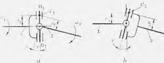
9.4-rasm. Teng bo'lmagan burchak tezlikka ega bo'lgan kardan sharnirining sxemasi
