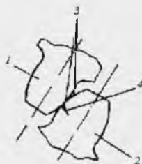
6.18-rasm. Tish materialining uvalanish sxemasi
