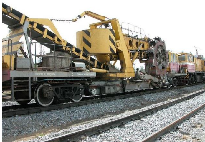
6.2-rasm. Ballast tozalash mexanizmi
