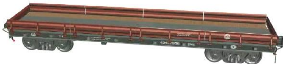
Rasm 10.3. Yaxlik metall bortli to‘rt o‘qli platforma
