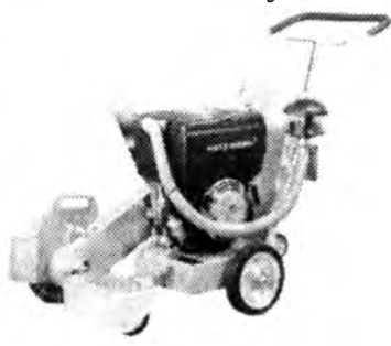
4.21-rasm. Choklarni tozalash uchun metall cho'tkali mashina
