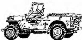
Fig. 16. The Jeep, built during and after World War II as a general-purpose vehicle with four-wheel drive
