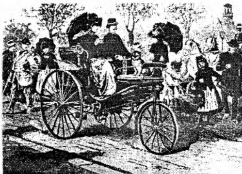
Fig. 1. A Benz tricycle, powered by an internal combustion engine
