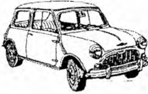
Fig. 18. The Mini: introduced in 1959, designed by Alec Issigonis with features such as front-wheel drive, transverse engine, and 10-in (25 cm) wheels
