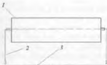
3.1.5-rasm. Noriya taranglovchi barabanini o'rnatish 1-taranglovchi baraban; 2-sohul; 3-polda chizilgan montaj o'qi
