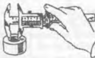
1.2.31- rasm. Shtangensirkul yordamida ichki diametrni o'lchash
