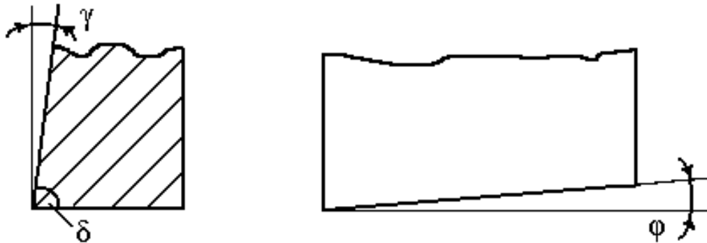
6.2-rasm. Qirqadigan pichoqning geometriyasi
