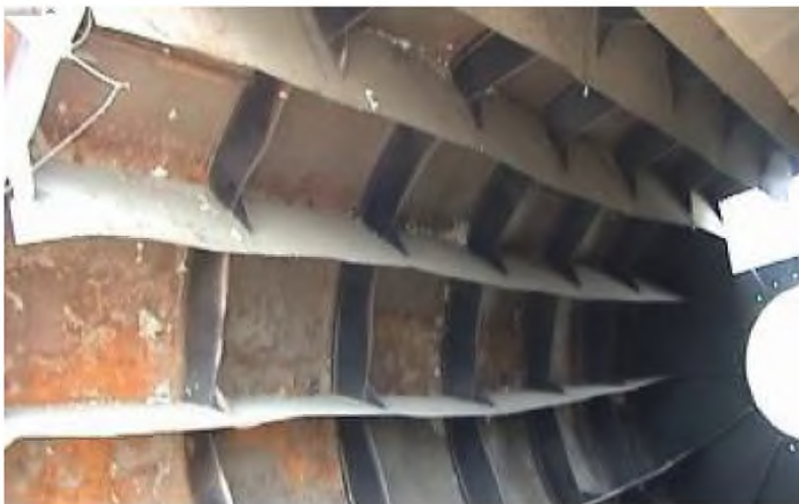
7.2-rasm. Quritish barabanining ichki qismi.
