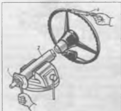
81-rasm. «ZIL-130» avtomobilining rul vali podshipnigini sozlash:
