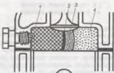
2.8-rasm. Ish aralashmasining yonish sxemasi:
