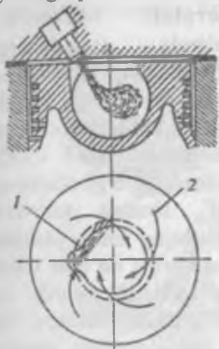
9.5-rasm. Purdali aralashma hosil qilinadigan kamera:
