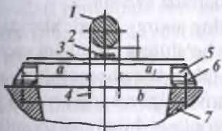
11- rasm. Statorni poydevor plitasida tekshirish (o'lchab ko'rish) sxemasi:
