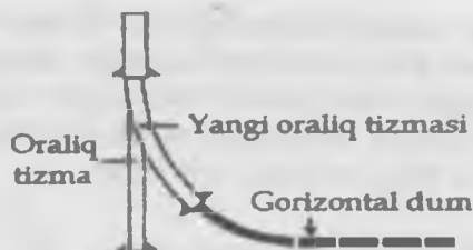
8.4-rasm. Oraliq tizmasida derazani ochish
