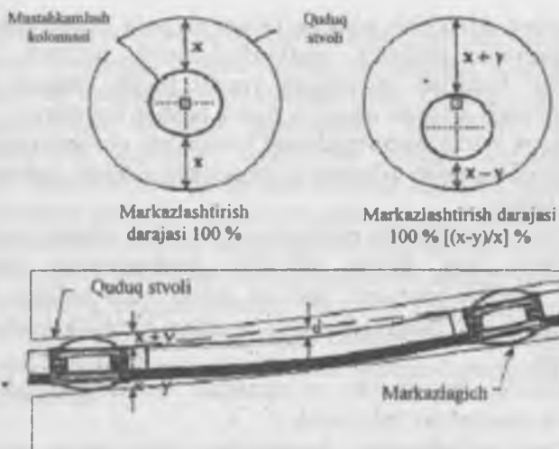
14.9-rasm. Mustahkamlash tizmasini markazlashtirish darajasi
