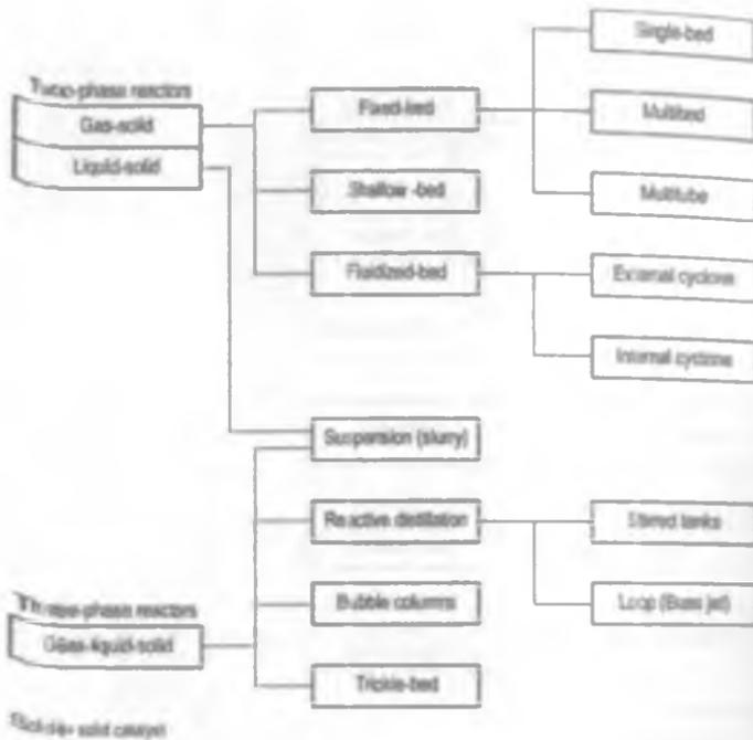
Figure 24. Classification of industrial reactors
