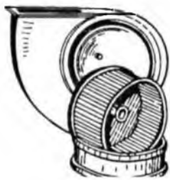
14-rasm. Markazdan qochma ventilator.
