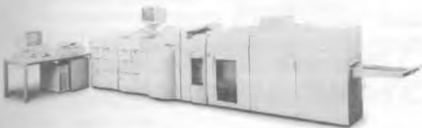
9.2.3-rasm. Potok liniyasida broshyuralar tayyorlash uchun bosma tizimi (elektrofotografik bosma usuli) (Digimaster 9110, Heidelberg)
