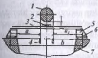
5.11- rasm. Statorni poydevor plitasida tekshirish (o'lchab ko'rish) sxemasi:
